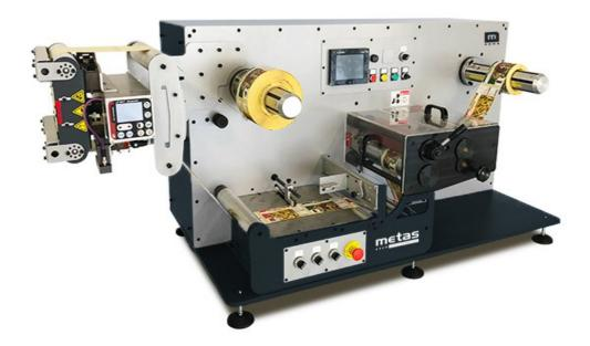
Metas Lite inspection Machine is a compact and highly efficient tabletop slitter rewinder machine. It has an accurate web tension control using manual clutch and brake. The machine is equipped with a splice table with pneumatic clamps for a quick and simple change of master roll, 3 sets of circular knives with lateral adjustment and razor knives as an optional. The Metas Lite inspection Machine is a cost-effective solution to slit, and rewind printed webs..
